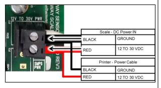
The power cable needs to be connected in the same connector as the DC supply wires. Make sure source power is disconnected to avoid shorting and damage.
