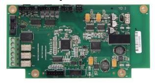
The Belt-Way Integrators I-O Option Board enables customers to increase the functionality of their belt scale controller.
